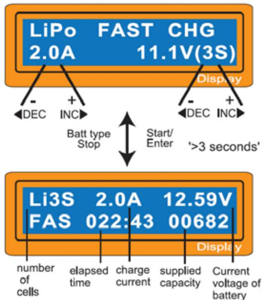
number of cells    elapsed time    charge current    supplied capacity    Current voltage of battery
